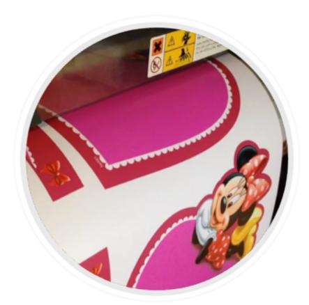
The foil used is synthetic paper that is 100% recyclable, waterproof and tree-free, using eco-solvent ink.
